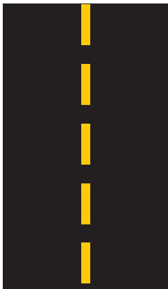
Broken line — passing is allowed when safe
